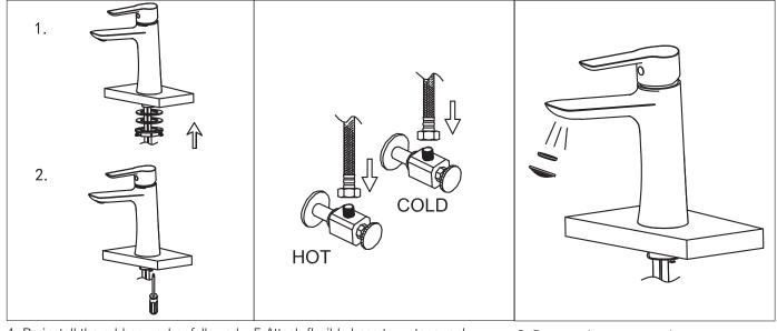
4. Re-install the rubber washer followed by the metal washer and lock-nut. Hand tighten then tighten further using a screw driver to tighten lock-nut screws.
